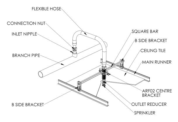
1. Install the Inlet Nipple in the branch pipe outlet using the normal sealing and tightening methods for connecting pipe threads. Tighten firmly with a pipe wrench for leak proof connection.
