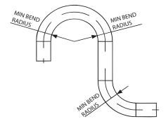
The flexible stainless steel hose should not be bent within 65 mm (2 1/2 inches) of its connection nuts
